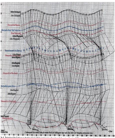
ig. 4. Projection of the 31 phases on the plane of gait with the partial centres of gravity (red), the centres of gravity of different systems (blue) and the total centre of gravity of the ody ( $\odot$ )
