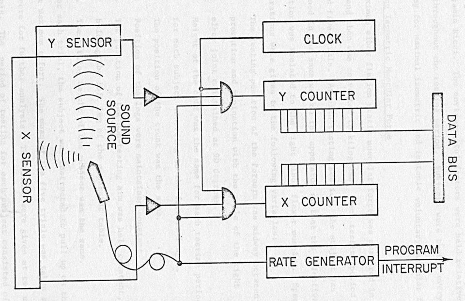
FIGURE 4. Schematic representation of Graf-Pen operation.
