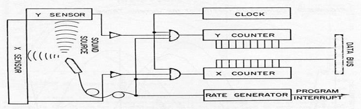
FIGURE I. Schematic representation of Graf-Pen operation.
